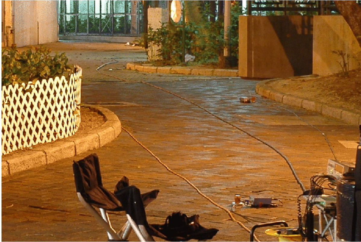
PHOTO 4 GEOPHONE ARRAY DESIGNED TO SIMULTANEOUSLY MEASURE VIBRATION LEVELS AT DIFFERENT LOCATIONS FROM IMPACTING POINT
