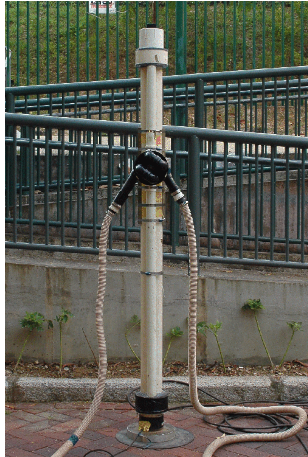
PHOTO 3 WHAMMY IMPACTING WITH A HAMMER PLATFORM SETUP ON THE GROUND TO TRANSMIT THE IMPACT FORCE TO THE TUNNEL
