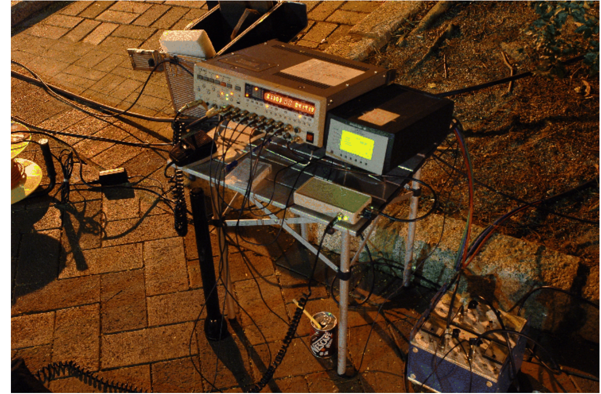
PHOTO 6 DATA ACQUISITION SYSTEM AND DIGITAL AUDIO TAPE RECORDER USED TO RECORD MEASUREMENT DATA
